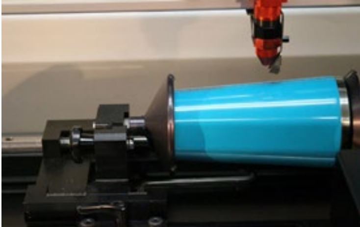
Use the X motion buttons to move the laser head to the center point
