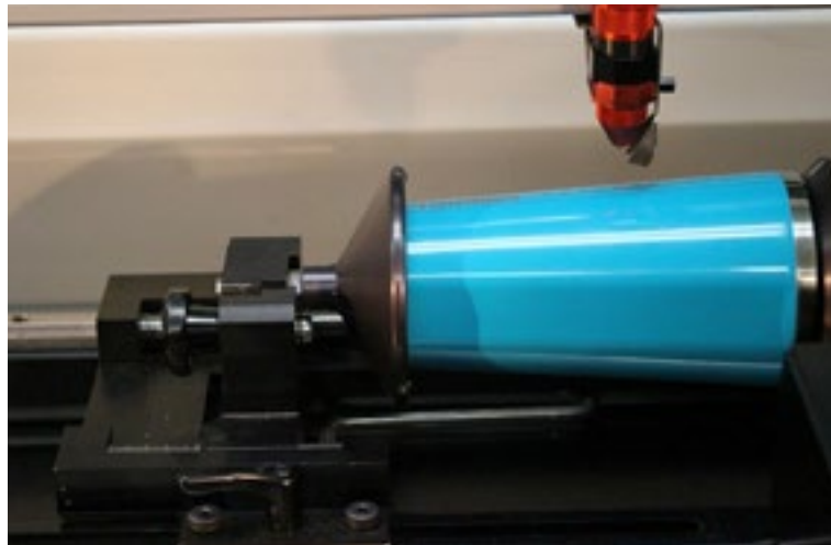
The mug can be loaded into the rotary fixture with the brand mark facing straight up
