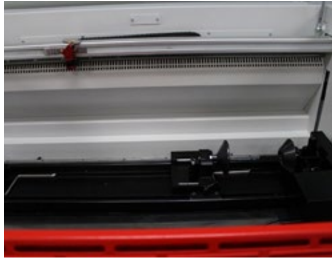
Place pointed cone to the right side of fixture to help with angle adjustment
